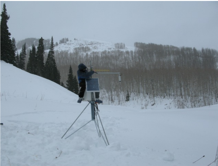
Grant, tweaking one of our snow depth sites in the 1000 Peaks Ranch.
